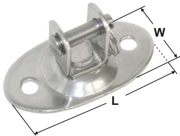
SWIVEL BASE stamped AISI 304 ITEM NO. L mm W mm Weight/g 005063 50 26
