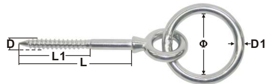
WOOD SCREW EYE RING AISI 316
